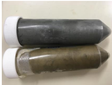
Figure 4. Subsamples of tailings from 77 m depth (grey, above) and 44 m depth (brown, below) showing the colour difference between the samples.
