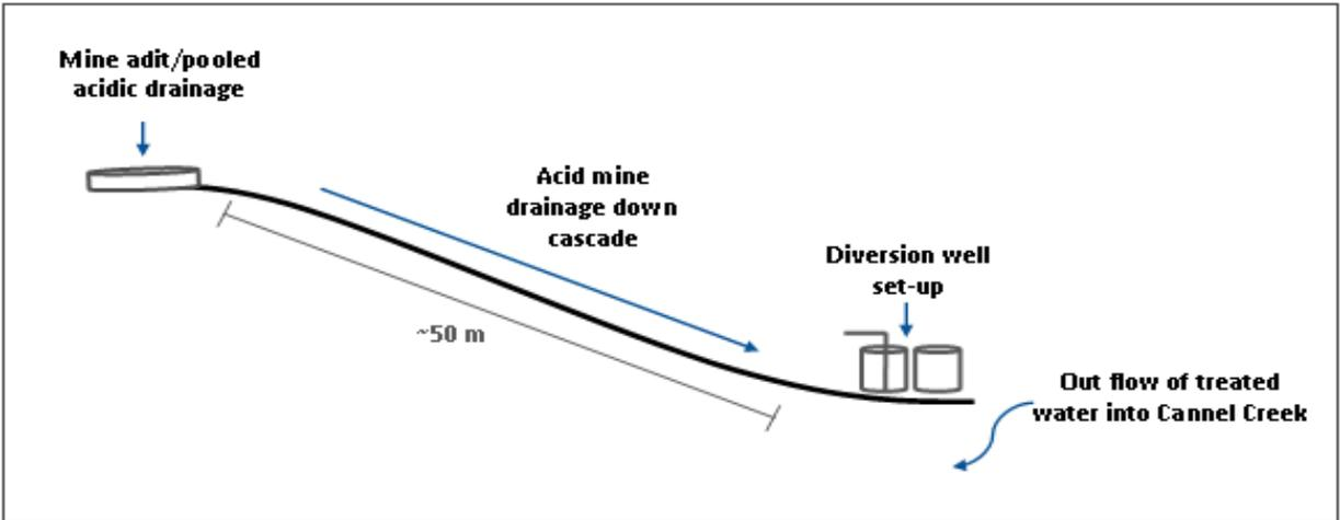
Figure 2. Schematic of Bellvue Mine site showing path of acid mine drainage (not to scale)
