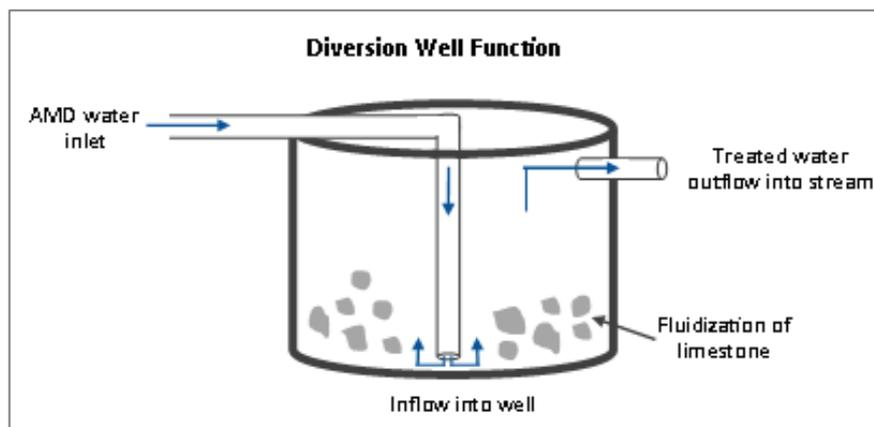
**Figure 3.** Schematic diagram of a diversion well design and function. Contaminated waters from an upstream dam flushed down central pipe into limestone substrate, allowing for neutralization of acidic water. Treated water is then flushed through an outlet pipe back into stream.
