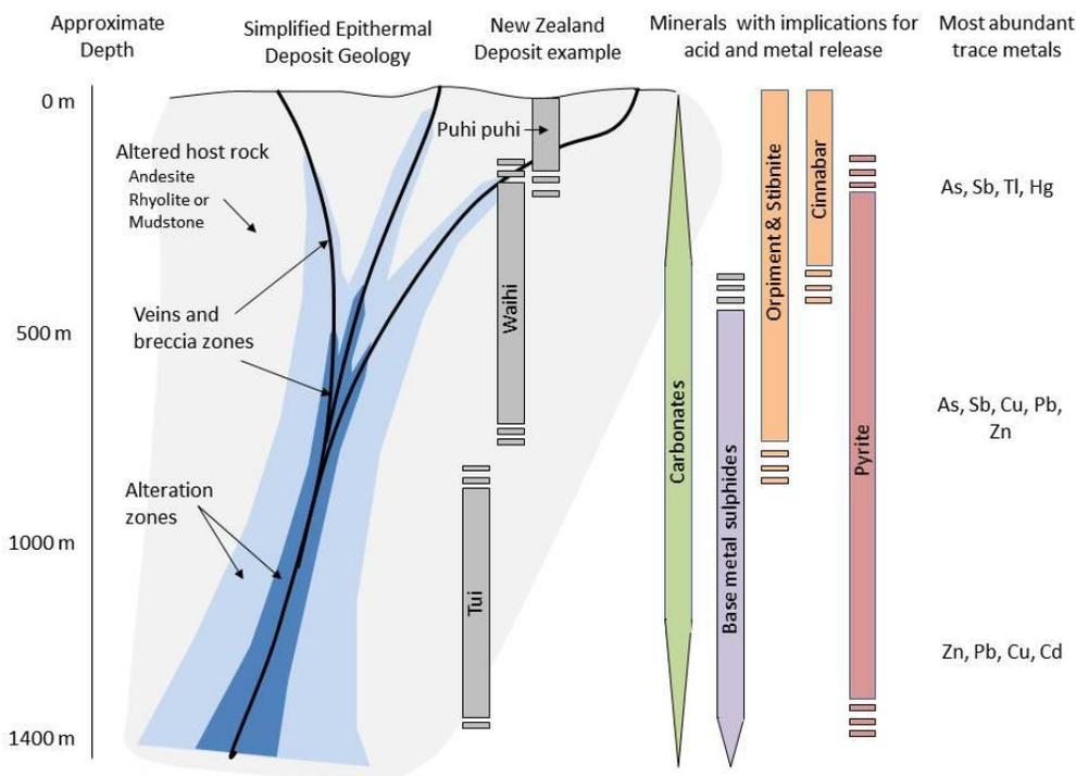
**Figure 2** Schematic of epithermal mineral deposit with a generalised model for the distribution of selected minerals that release or neutralise acid or contain trace elements.
