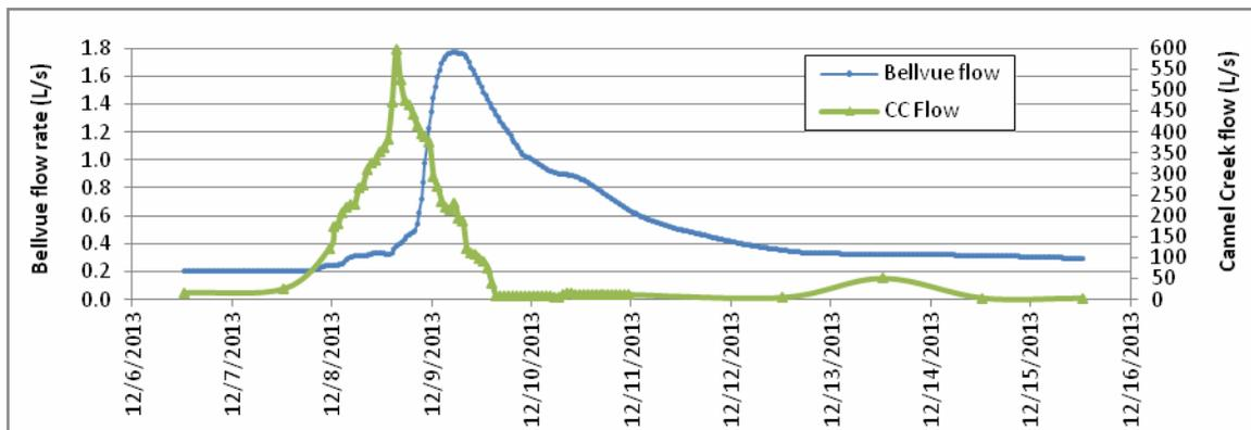
Figure 3. Example of asynchronous flow pattern between the Bellvue AMD and Cannel Creek.
