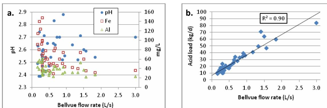
Figure 4. Bellvue Mine AMD a. Chemistry, b. acid load.
