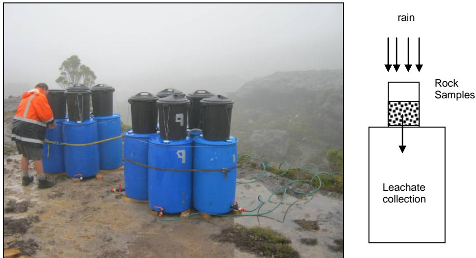
Figure 1: Lysimeter (field column) setup
