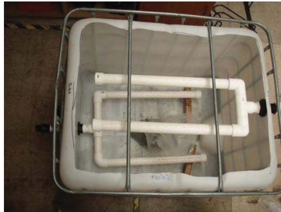
Figure 1 Adsorption chamber prior to being filled with treatment medium
