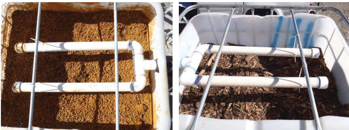
Figure 2 Adsorption chamber (on left) and bioreactor (on right) prior to being filled with water
