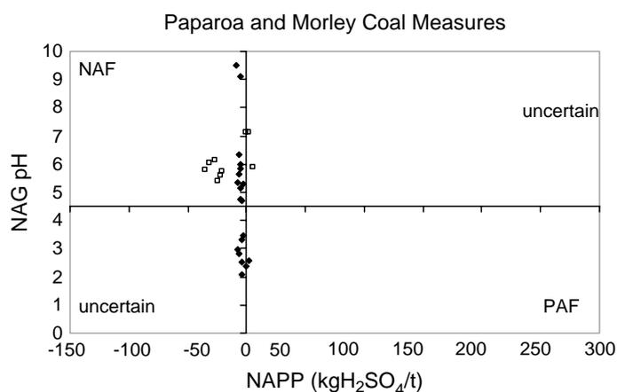
**Fig. 5** Comparison of NAG pH to NAPP acid producing potential for Paparoa (diamonds) and Morely (squares) Coal Measures. PAF—potentially acid forming, NAF— non-acid forming.
