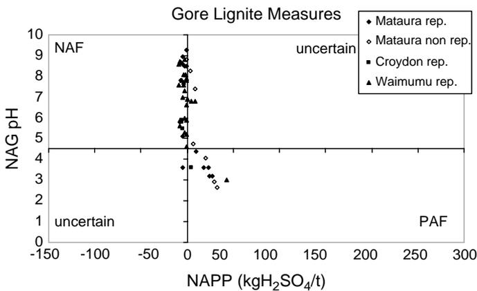
**Fig. 6** Comparison of NAG pH to NAPP acid producing potential for the Gore Lignite Measures. PAF—potentially acid forming, NAF—non-acid forming.
