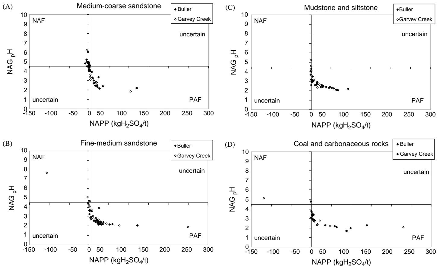
**Fig. 3** Comparison of NAG pH to NAPP acid producing potential for different rock types in Brunner Coal Measures rocks at Buller and Garvey Creek Coalfields. (A) Medium-coarse sandstone; (B) Fine-medium sandstone; (C) Mudstone and siltstone; (D) Coal and carbonaceous rocks. PAF—potentially acid forming, NAF—non-acid forming, uncertain—additional study required to determine acid producing/neutralising characteristics.
