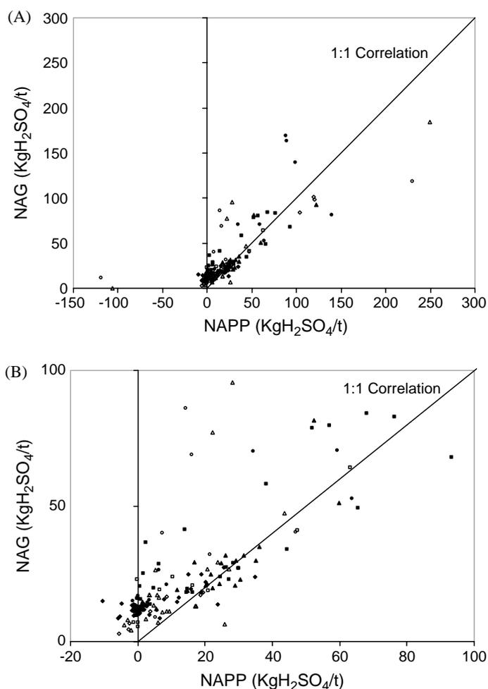
**Fig. 4** (A) Comparison of NAG acid production potential to NAPP acid production potential at Buller (closed symbols) and Garvey Creek (open symbols) Coalfields. (B) Scale up of axis region of Fig. 4A. Diamonds—medium-coarse sandstone, triangles—fine-medium sandstone, squares—mudstone-siltstone, circles—coal and carbonaceous rocks.
