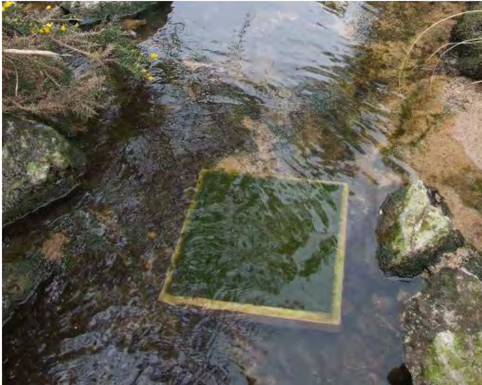
Plate 4.2: Artificial moss addition in T69. Astro turf simulating moss was glued to concrete paving tiles.
