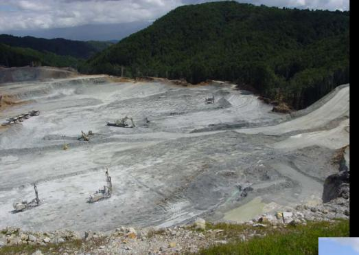
Mine excavation: ore contains As minerals As dissolves in runoff
